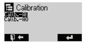
After calling up the calibration menu ("Calibration AI"), an overview mask of all analogue inputs is displayed. In addition to the input designation, the current measured value ("log.") and the converter raw value ("phys.") are displayed.
