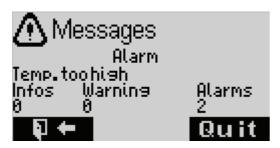
Current Alarms, Warnings and Infos can be selected and acknowledged (depending on the desired software setting).
