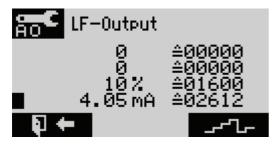
All values that are changed in the hardware diagnostics reset the control unit when exiting the menu.
