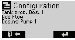
The module/function to be activated/deactivated is selected using the  $\Lambda/\Psi$ -buttons and set to either "yes" or "no" for the module / function to be activated.
