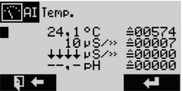
The input to be calibrated is selected with the aid of the  $\hbar/\Psi$ -keys and branched to the following calibration mask. Here, the current measured value as well as the lower and upper calibration point are displayed as logical as well as converter raw value.
