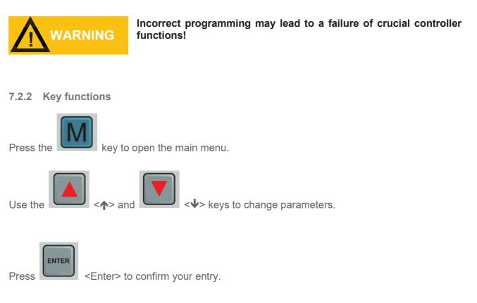
If you are entering parameters, pressing <Enter> will cause the cursor to move one position further right. If you are changing parameters, use the arrow keys to select the requested digit and then press <Enter> to confirm. Select all the parameters to apply the values.
