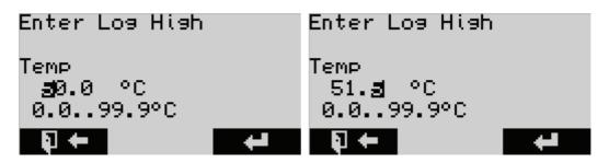
Change the value with the keys  $\uparrow$  or  $\checkmark$ , with **Enter** a digit is moved to the right. After entering the value, exit the mask with **Enter**.
