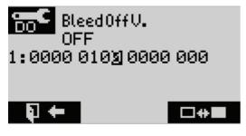
The analogue outputs can be selected with the  $\hbar/\Psi$ -keys, as with the digital inputs or outputs. Manipulation is possible via the **Enter**-key.
